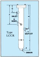
These models are available for installations up to 600 PSIG and temperatures to 100°F. Also available for steam service up to 500°F.
